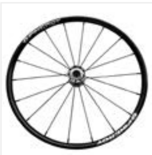
// QSF070005 Rear wheel, Spinergy, 18 spokes (black), straight spokes; hub: silver
